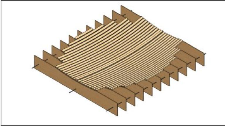
*Figure 4: Scheffler disc construction method.
