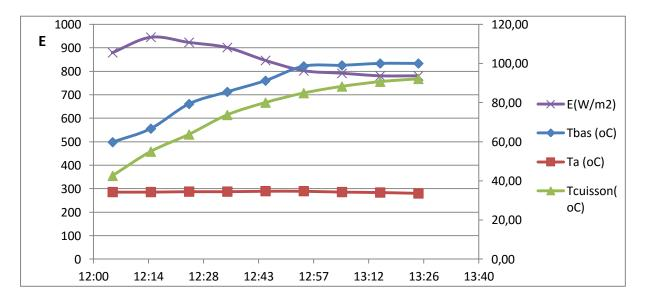
Figure 4. Temperatures and solar radiation evolutions for cooking with glass cubic box
