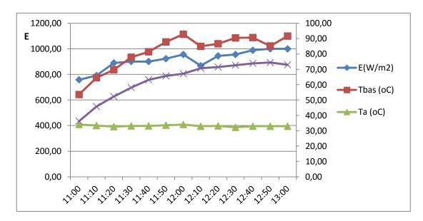
Figure 4. Temperatures and solar radiation evolutions for cooking without glass cubic box
