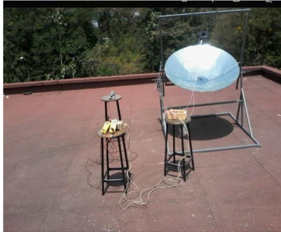
Figure 3. Experimental device with the ellipsoidal concentrator
