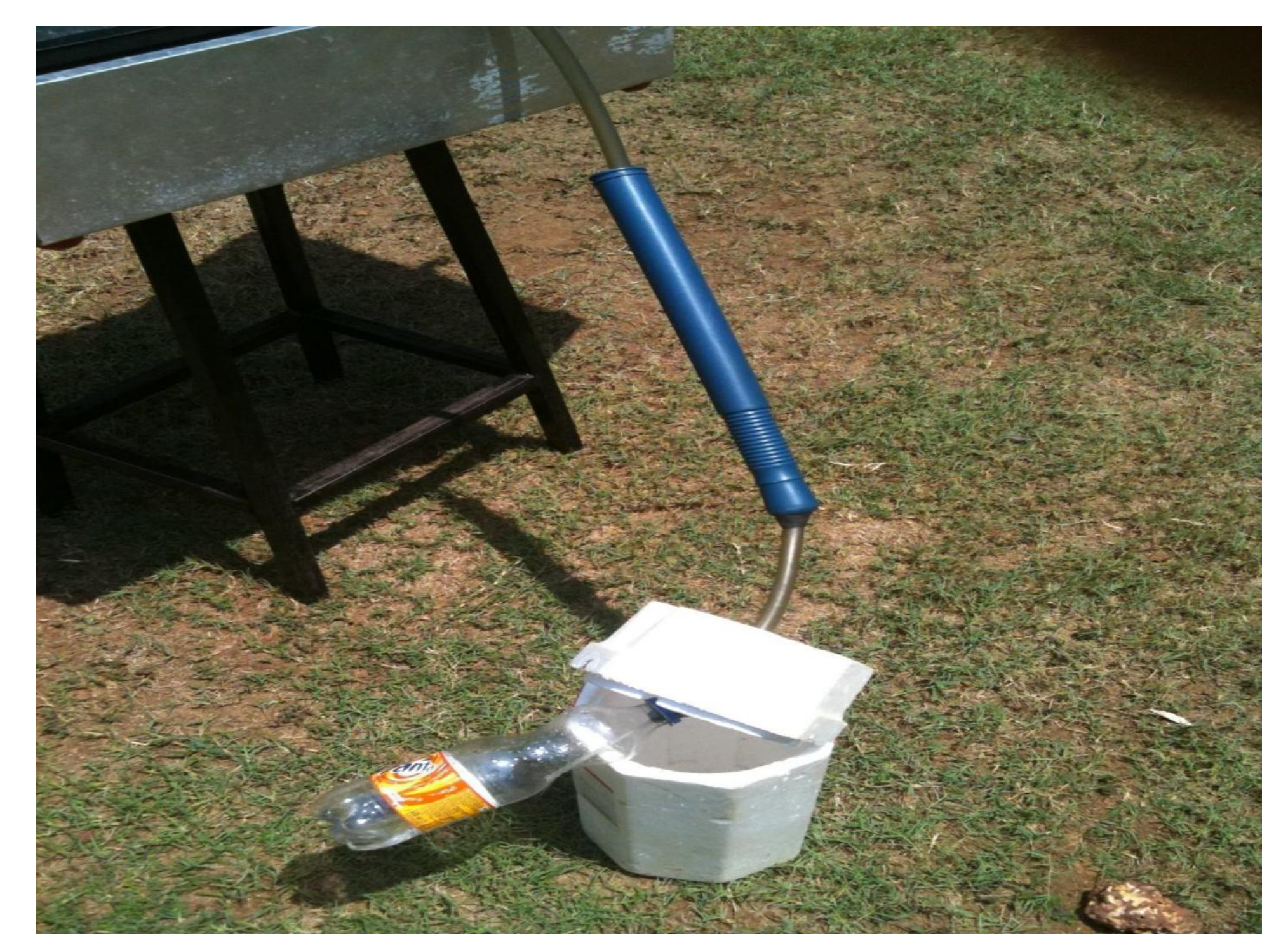
Fig.5. Condensation column with bottle as the collecting point of the Distillate
