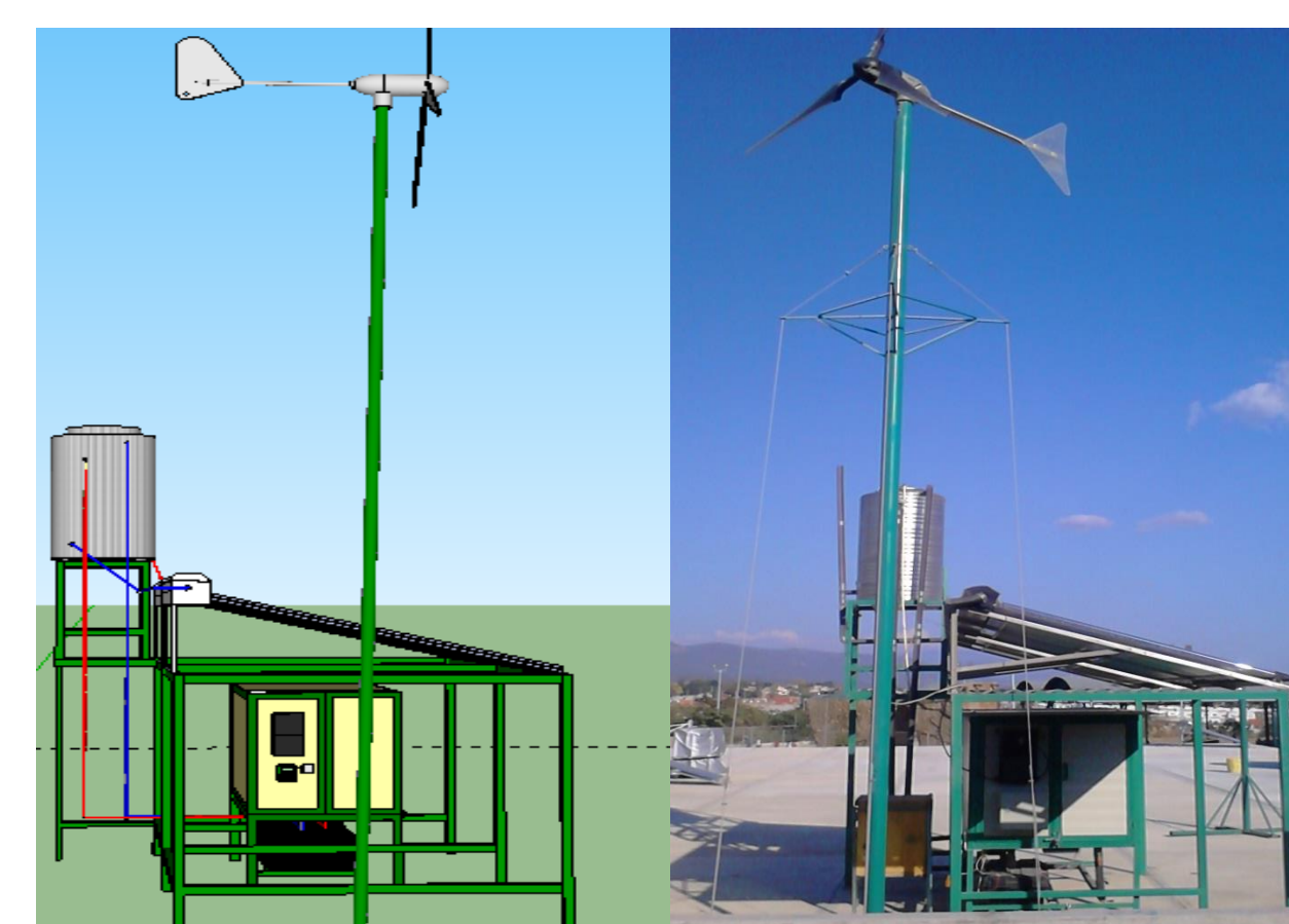
Figure 2. Hybrid dryer in solar platform - CIDTER, UNICACH, Chiapas, MX.
