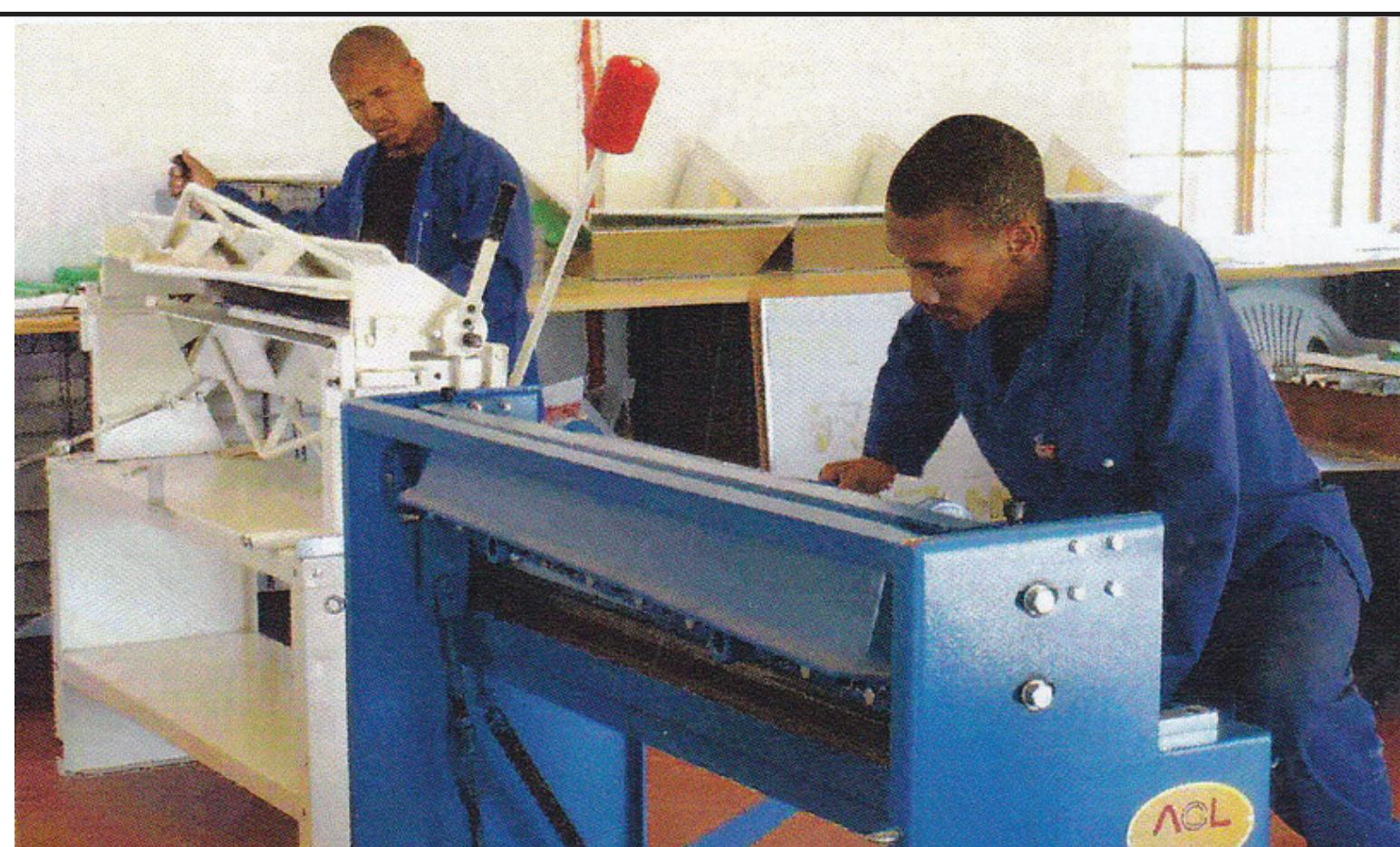
The cooker production requires a guillotine shear (left), a sheet metal bender (right), a circular saw and a hand-drill.
