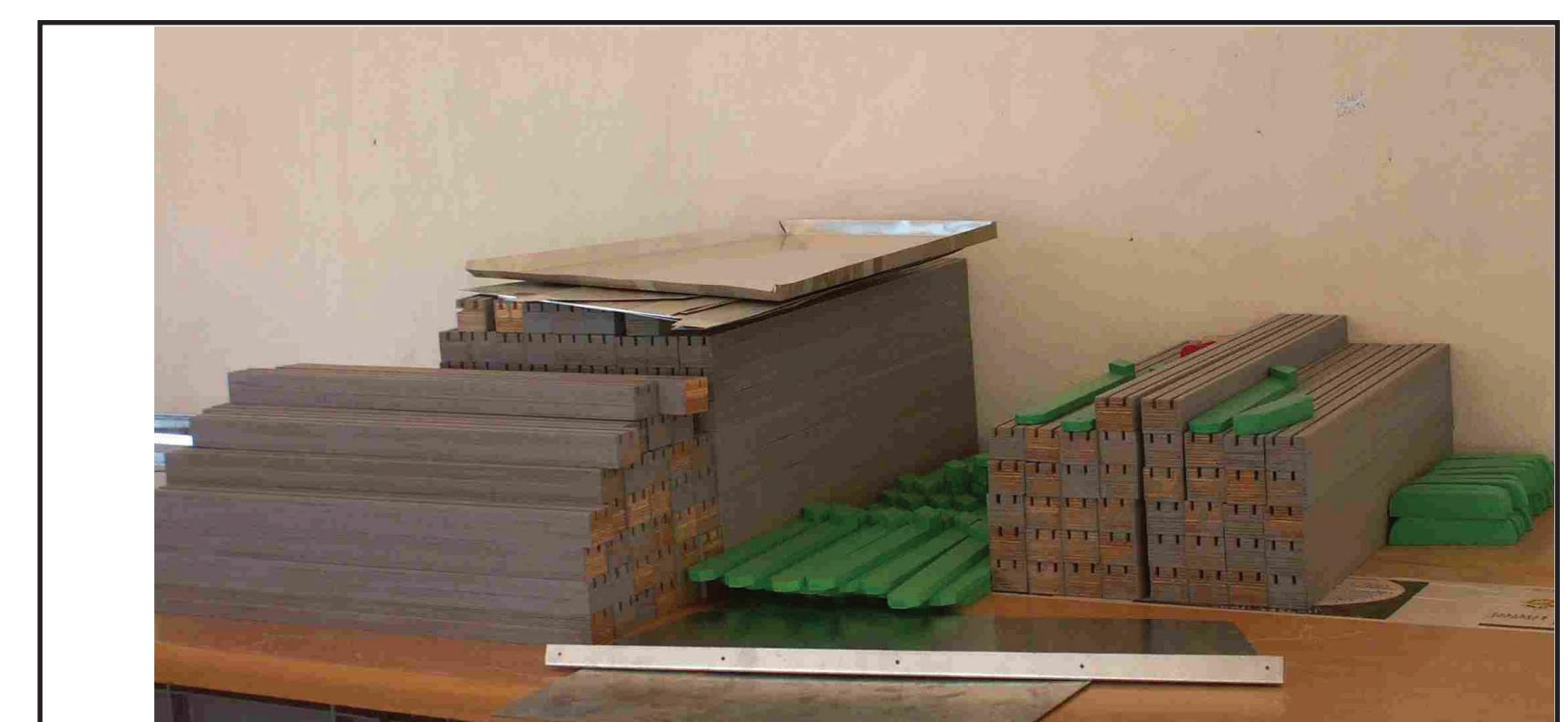
The manufacturing concept is aimed for serial production. Every step is standardized. As all work is supported by templates and jigs, measuring and marking are mostly obsolete.
