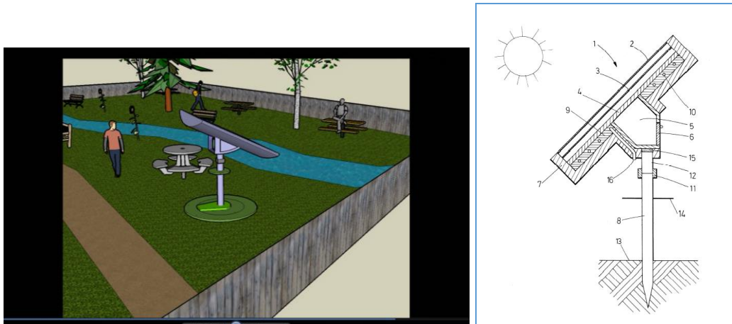
Figure 1. (left) Solar cooker rendering, shown in a park. A step allows reaching the oven door. A shelf facilitates cooking manoeuvres and ingredients storage. The height avoids children damage. (right) cross cut of the design, including extra heat storage below the absorber plate and the capability of heating water for cleaning.
