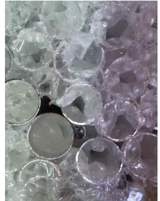
PCM retraction when solidifying.
